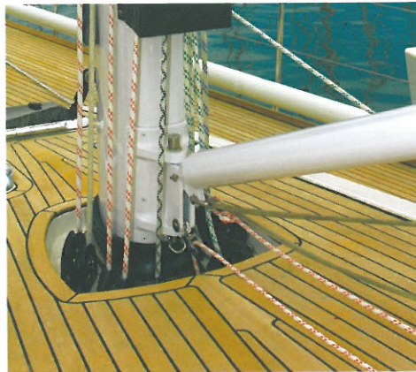
Control and trim lines led under deck
