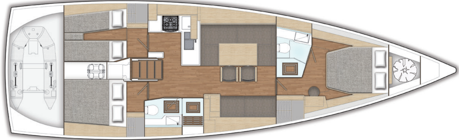
Optional Layout - double & twin cabins aft, aft facing chart-table with dedicated shower compartment in the aft heads
